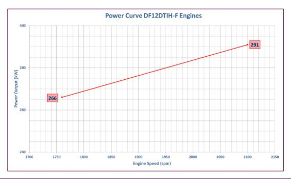
Although our FM ratings are shown at specific speeds, De Maas FFE engines can be applied at any intermediate speed. To determine the intermediate speed power; make a linear interpolation from the applicable De Maas power curves.
