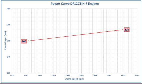
Although our FM ratings are shown at specific speeds, De Maas FFE engines can be applied at any intermediate speed. To determine the intermediate speed power; make a linear interpolation from the applicable De Maas power curves.
