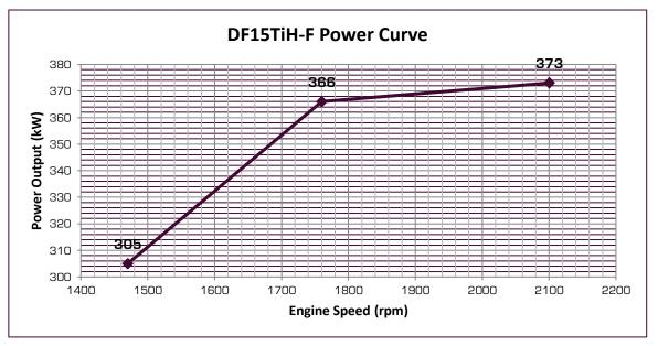
Although our FM ratings are shown at specific speeds, De Maas FFE engines can be applied at any intermediate speed. To determine the intermediate speed power; make a linear interpolation from the applicable De Maas power curves.
